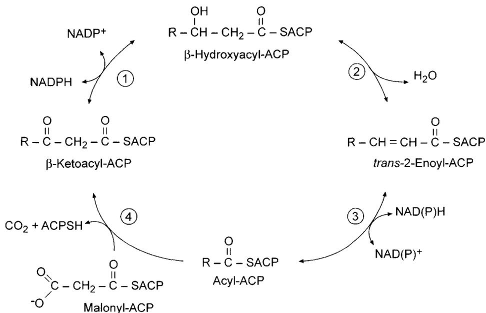
Fig. 3. Cycles of fatty acyl chain elongation. All intermediates in fatty acid synthesis are shuttled through the cytosol as thioesters of the acyl carrier protein (ACP). (1)  $\beta$ -Ketoacyl-ACP reductase (FabG). (2)  $\beta$ -Hydroxyacyl-ACP dehydrase (FabA or FabZ). (3) *trans*-2-Enoyl-ACP reductase I (FabI). (4)  $\beta$ -Ketoacyl-ACP synthase I or II (FabB or FabF).
